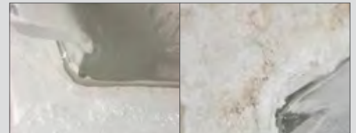
Adhered surface contamination cannot be repaired.
