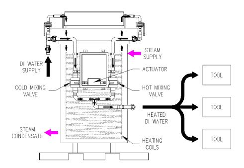
The overall pressure drop across the system remains nearly constant, regardless of the position of the mixing valves, due to the fact that as one of the mixing valves is opening, the other is closing, so the combined cross-sectional area of the two valves is essentially constant.
