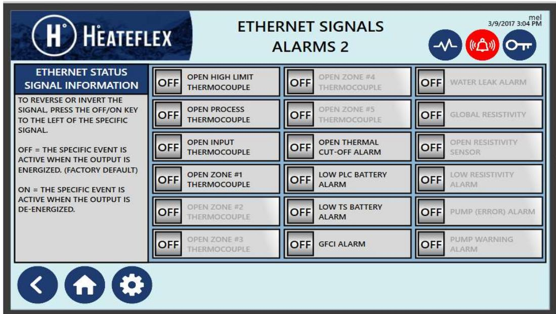
**Figure 18-10: Ethernet Signals Status Screen**
