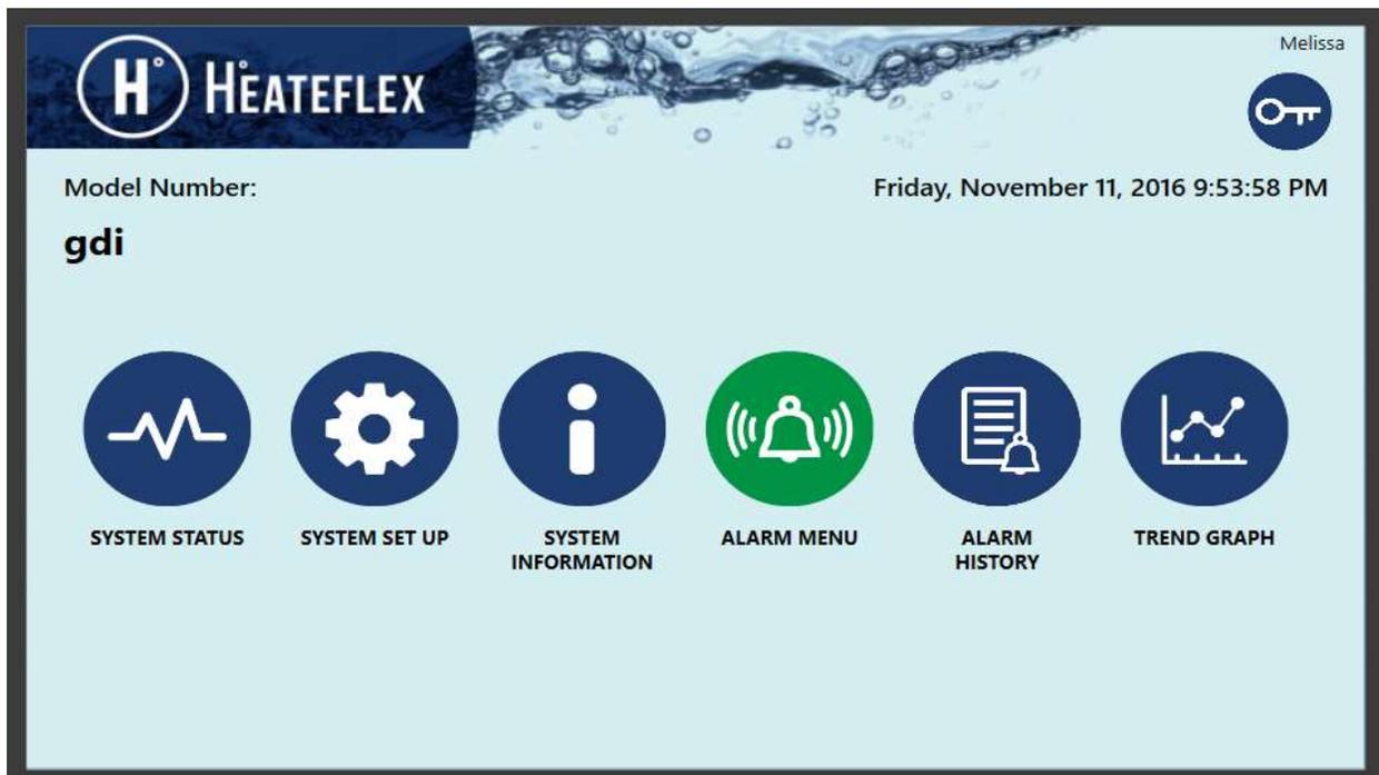
The **System Set Up Menu** (See Section 6.1) is used to access system settings and troubleshooting. These settings include **Control Settings**, **Alarm Set Points**, **System Calibration**, **Factory Setup**, **Ethernet Interface**, and **Option Settings**. Note: A factory password is required to access the **Trouble Shoot Menu** and **Factory Set Up Menu**.
