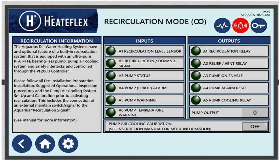
This pump air cooling system calibration is achieved by regulating the air pressure of the pump air cooling system when it is active. To perform this calibration procedure access to the interior enclosure of the Aquarius® D.I. Water Heating System with the system powered ON is required.
