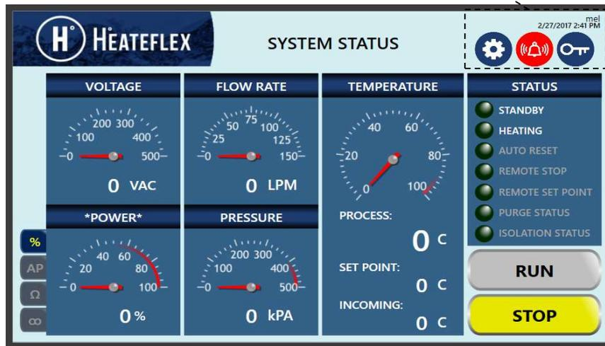
The password is eight digits alpha-numeric. This password will allow the user to modify the parameters and set points within the **Control Settings**, **Alarm Set Points**, **System Calibration**, and **Options** (if options are available). In addition, the **User Password** is required in order to clear the information on the **Alarm History** screen and in order to activate the **GFCI TEST** key for the **GFCI Alarm**.
