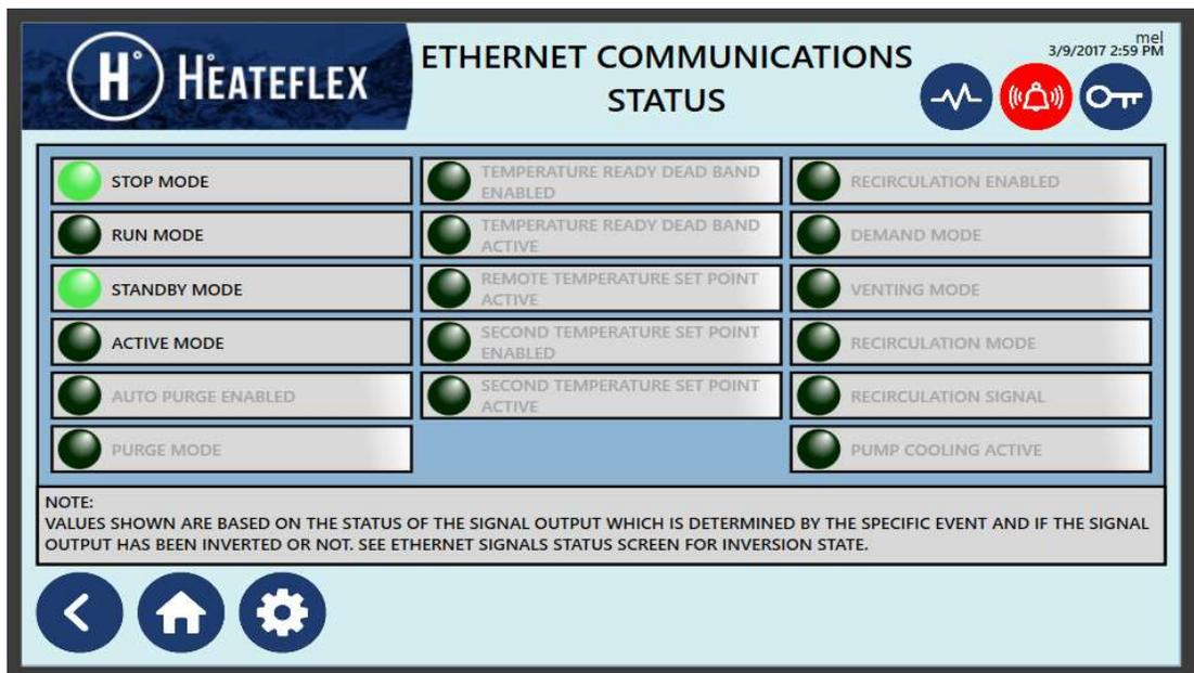
Note: This screen indicates that the system is in “**Stop**” mode and “**Standby**” mode.
