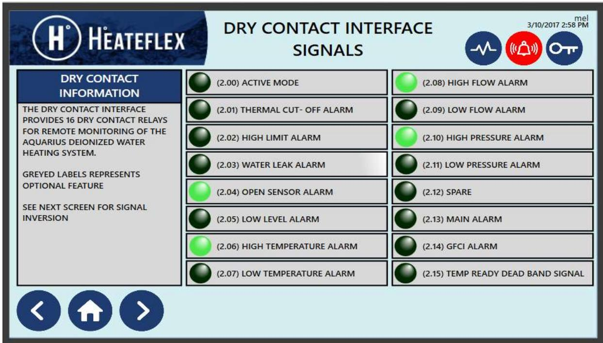
Figure 17-2: Dry Contact Interface Signals Screen #2
