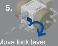
**5.** Move lock lever to down position. Reattach L bracket. Tighten hand tight.
