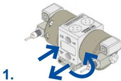
**1.** Set lever to up position. Slide base plate forward or pump body backward.
