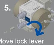
**5.** Move lock lever to down position. Reattach L bracket. Tighten hand tight.
