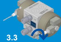
**3.3** Move lever down to locked position.
