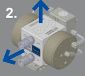
**2.** Slide pump forward; lift it off base plate.
