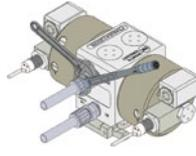
**6.** Attach tubes and fittings per manufacturer instructions. Use backer wrench to hold fitting in place at pump.
