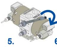
**5.** Attach fittings to pump. Tighten to 55 inch-lbs.
