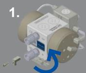
**1.** Remove L bracket. Set lever in neutral (up) position.
