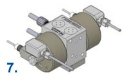
**7.** Set air line via 1/4 in FNPT ports on quick exhaust valves. Line must be 1/4 in minimum orifice.
