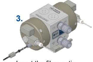
**3.** Insert the fiber optic cable until it contacts the bottom of the probe.
