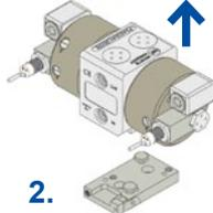
**2.** Lift pump off of base plate.
