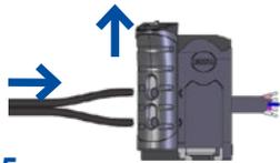
**5.** Open the top and slide the front face of the D10 up. Press the fiber optic ends into the holes on its front. Slide the face down to lock cables in place.
