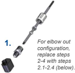
**1.** For elbow out configuration, replace steps 2-4 with steps 2.1-2.4 (below).
