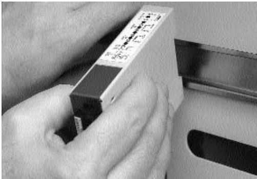
Step 1: Orient the controller so that the wiring label is visible after the unit is attached to the DIN rail.
