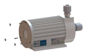
1. Remove the three fastener cover caps and 5/8-inch length, 10-32 fasteners from back of pump.
