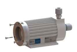
Place air-cooling module on back of pump and secure with 1.5-inch length 10-32 fasteners.
