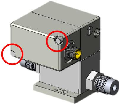
To switch the operation mode of the PPMC300, the electrical cover will need to be removed. To remove the cover, remove the cap screw covers and the two cap screws that hold the electrical cover in place (shown in image to the left). Once the cover has been removed find the surface mount potentiometer on the circuit board (Shown in image to the right). Use
