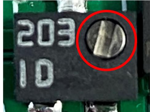
a small flathead screwdriver and rotate the potentiometer to the desired position. Rotating clockwise will decrease the cycle rate, and rotating counter-clockwise will increase the cycle rate.
