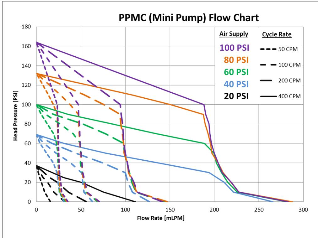
\*300 mL/min at wide open flow path. The Flow Chart measurements shown are using a back-pressure regulator to simulate a pressurized system; results may vary.
