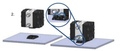
Attach base plate to work space using 4 bolts, in predrilled holes. Align pump to base plate and lower onto stand, ensuring base is fully seated. Tighten set screws on front of base.
