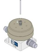
Attach air-line to device. Min 1/8in ID tubing.
