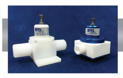
The relief valve is fully adjustable within this range by simply adjusting the upper Socket Hex Adjustment Screw and locking in place with the associated locking nut.
