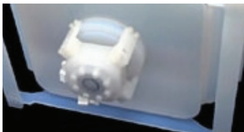
PFA tank, dump door, and mounting ring with NPP valve body. Custom PFA tanks are common for quick dump rinsing steps.
