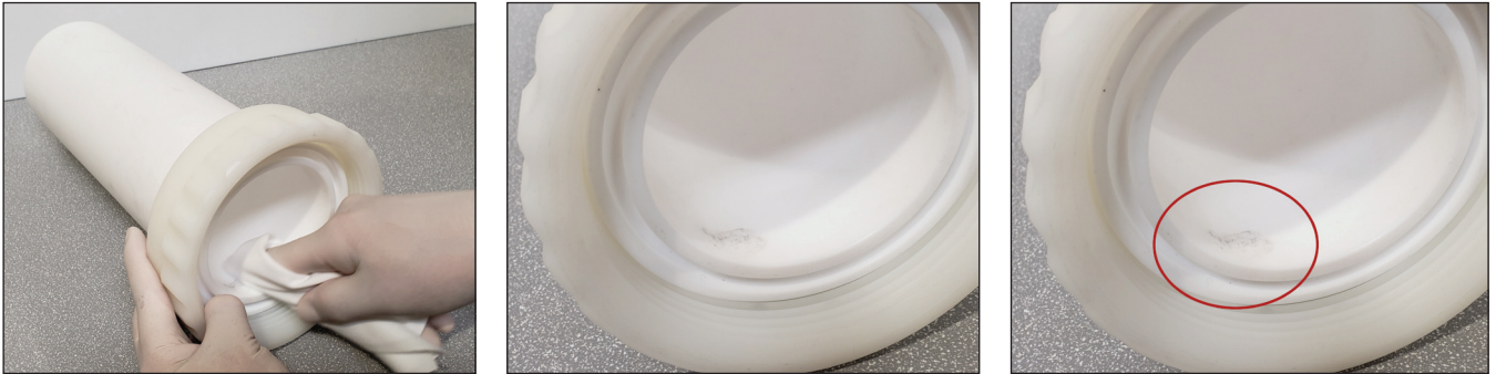
Figure 4. PTFE compression-molded/machined housing after wiping with a dry paper towel. Pigments from the liquid marker remain embedded in the material
